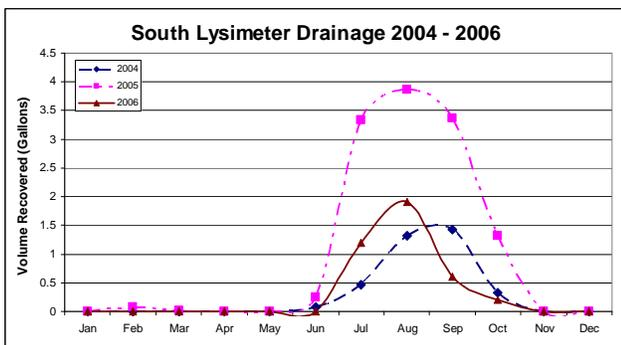
**Graph 9 – BCSL South Lysimeter Recorded Drainage**
